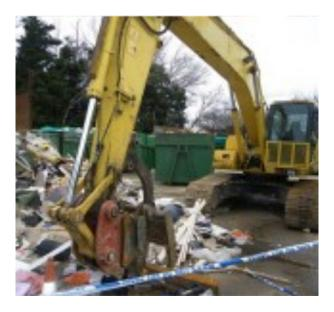
A company director was operating a 3600 tracked excavator, which he was using to transfer waste from a main pile to an adjacent manual-sorting area. The injured worker moved behind the excavator to pick up an old door and place it in a skip. As he did so, the operator reversed the plant, crushing the worker beneath one of the tracks. He sustained serious crush injuries to his right leg which later required amputation in hospital.
