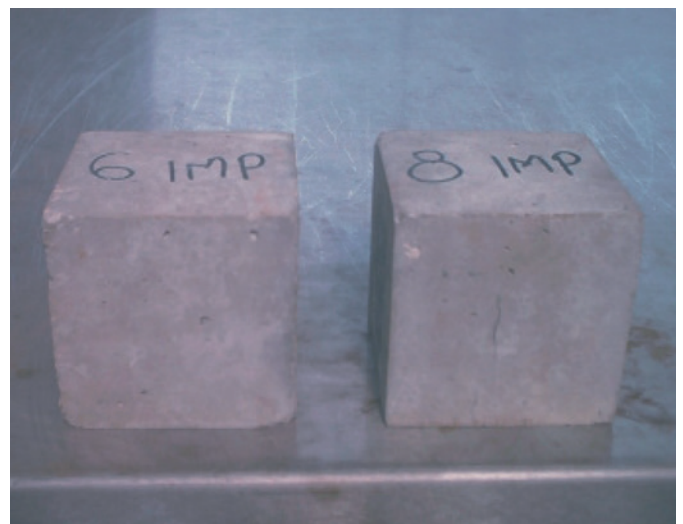
Concrete treated with Vetrofluid and subject to 300 freeze-thaw cycles
