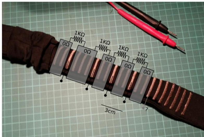
**Figure 2. Stitching thread in the Smartcap band and their conductivity relationship.**
