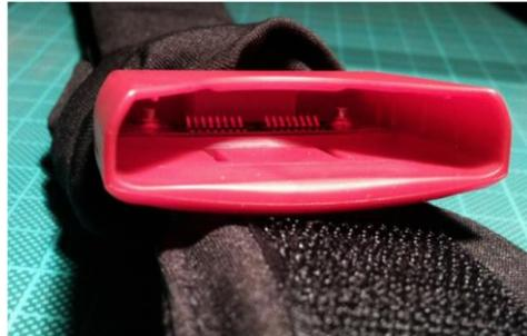
**Figura 3.** The band has a receptacle connector (16 pins) for the Smartcap processing unit.
