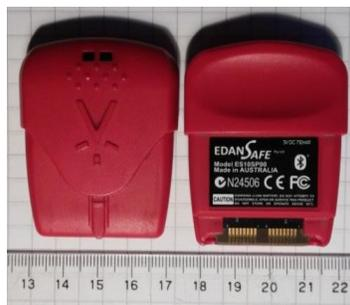
**Figure 4.** Smartcap processing unit that encapsulates CPU, battery and Bluetooth communication module.
