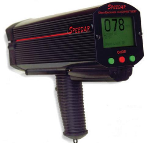
Speedar is a handheld speed and direction measuring Doppler radar, with large backlit 128x64 dot graphic display. Capable of measuring speeds in Miles or Kilometers per hour and displaying system messages in any language.
